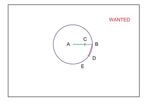
Set the compass to distance AC and draw the circle with centre B and distance AC.
