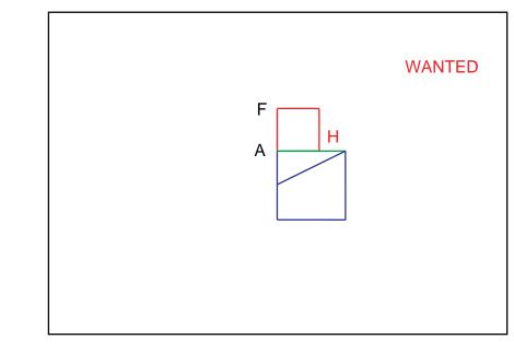
Swing from the corner, A. Locate the point H on AB so AH is equal to AF. (or, dividers.)
